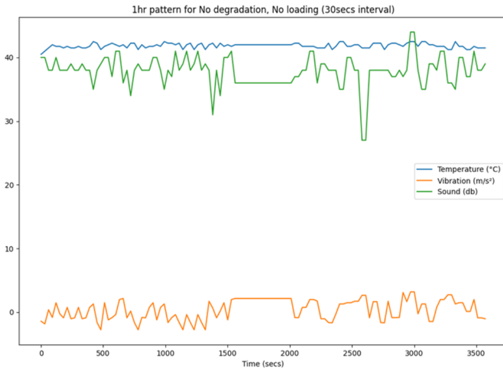
Figure 8 | Monitoring spectral for the rotary dryer under normal at no loading state
