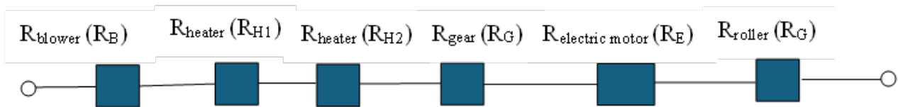
Figure 3 | The series reliability diagram for plantain rotary dryer
